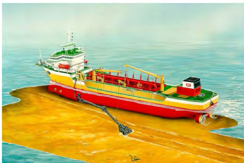
Figure 7: Trailing Suction Hopper Dredger (TSHD) (Source: IHC (Artists impression))
