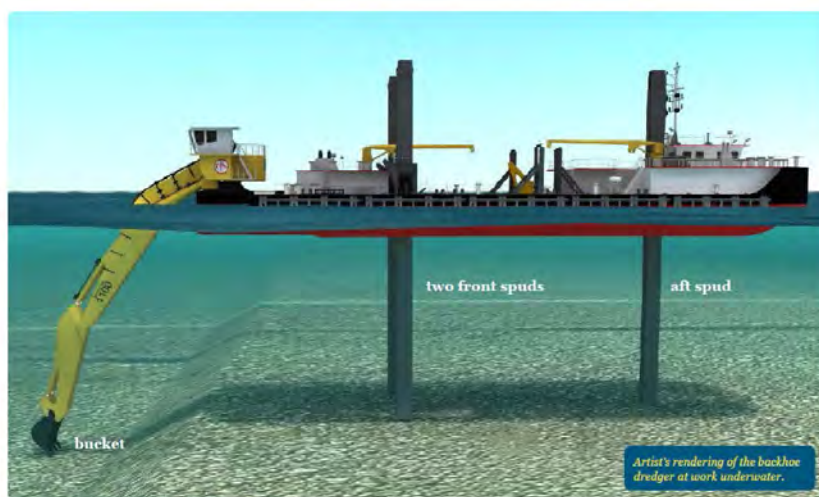
Figure 12: Backhoe Dredger (BHD) Source: IADC, 2016
