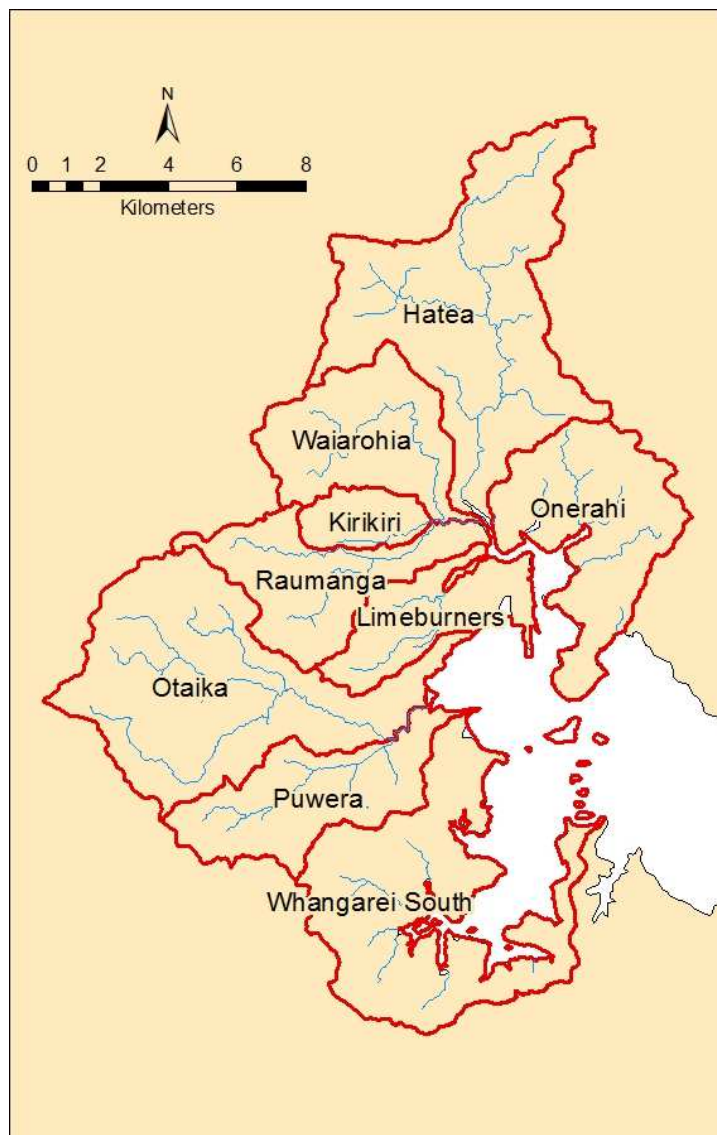
Figure 2-2: Sub-catchments of upper Whangarei Harbour.
