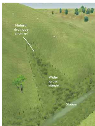
Figure 5: Using grass margins to filter channelled runoff.
