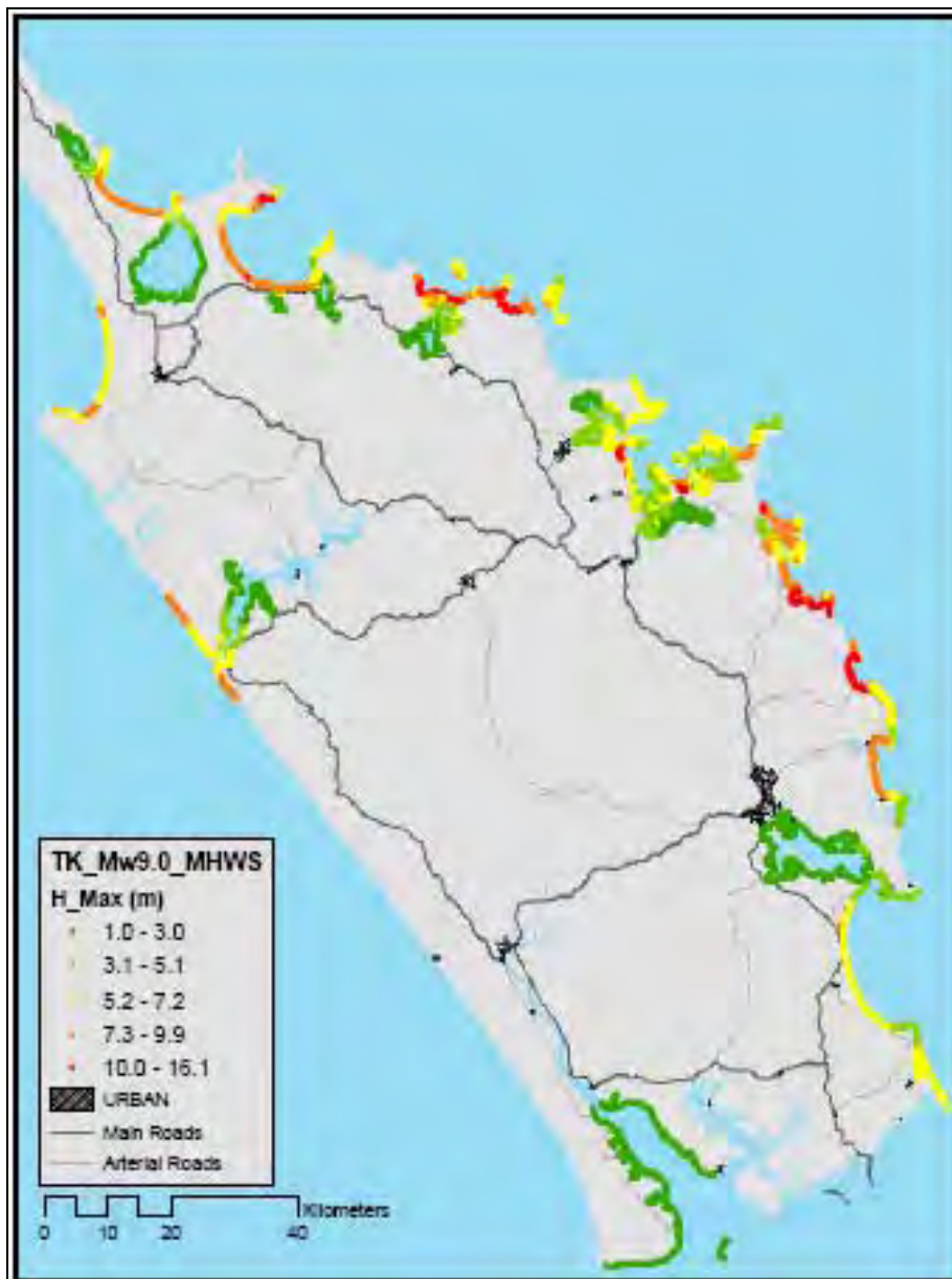
Map: Maximum wave height at shoreline for the Mw9.0 Tonga-Kermadec subduction zone scenario at MHWS. Areas of shoreline with no colour were not included in the model output.
