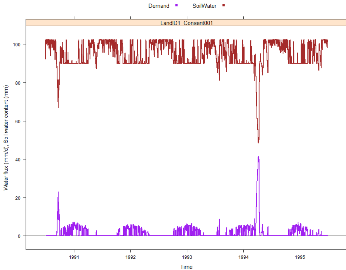
Figure 3-8: Calculated time-series of irrigation water demand and soil water content under the five-band harvesting experiment for July 1990 to June 1995.
