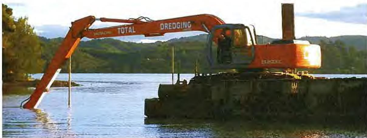
Figure 5: Total Dredging Ltd.'s Longreach excavator and hopper barge
