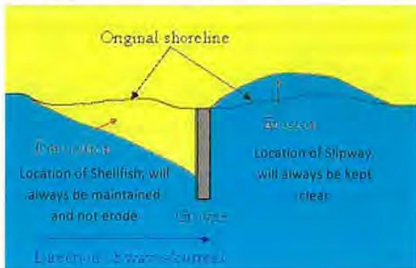
Figure 6: Illustration of how a groyne works
