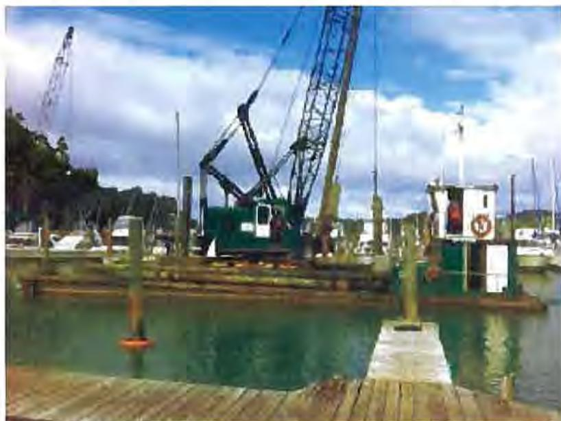
Figure 7: 50t Piling barge 'Northland Piler'
