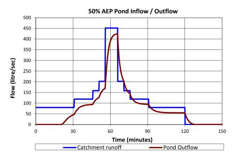
Attenuation provided by the ponds will be much greater in frequent, lower intensity rainfall events because a larger proportion of runoff is able to soak into the subsoil below the pond. One third of the existing 2 year ARI flow is the flow adopted by Auckland Council GD01 and TP10 for controlling erosion and sedimentation and is termed the water quality volume (WQV). It accommodates 95% of rainfall events, but excludes extreme rainfall events (10 and 100 year ARI).
