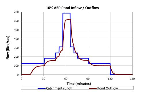
It can be seen that in a 10% AEP rainfall event, peak runoff is reduced by around 10%, but there is little delay in the discharge.
