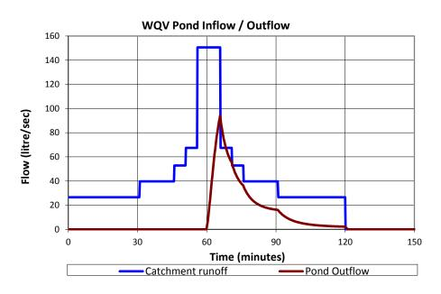
As noted in Section 6.7.3 of the Report, the existing pond upstream of the new 1800mm diameter culvert on the Hall Road access provides only minor attenuation of stormwater runoff from the site. However, and more importantly, it does not delay the release of stormwater to the stage where it may affect peak flows in the tributary.
