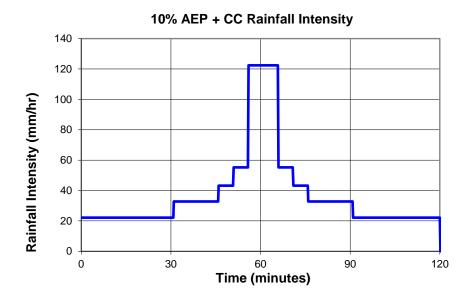
Stormwater runoff has been calculated using the Rational method. A soakage rate of 200mm/h has been assumed in the model.
