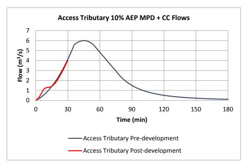
In each case, the changes to stream flow are minor and occur at the early stages of a flood event so do not add to peak flow.
