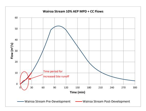
It can be seen from the graph that the increase in runoff from the site at the early stage of flood flows in the Wairoa Stream will have no effect on peak flows in the stream.
