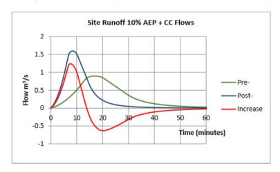
The effect of the increased site runoff to the Wairoa Stream upstream of the tributary junction for the 10% AEP + CC rainfall event is illustrated below:
