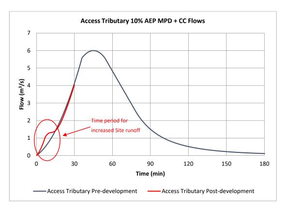
It can be seen from the graph that the increase in runoff from the site at the early stage of flood flows in the Tributary will have no effect on peak flows in the stream.
