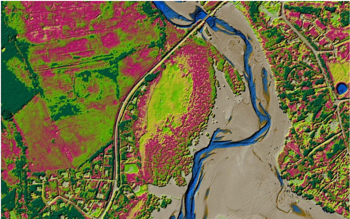
Figure 2: Normalised differentiated vegetation index raster layer, using the equation NDVI = (NIR - red) / (NIR + red)
