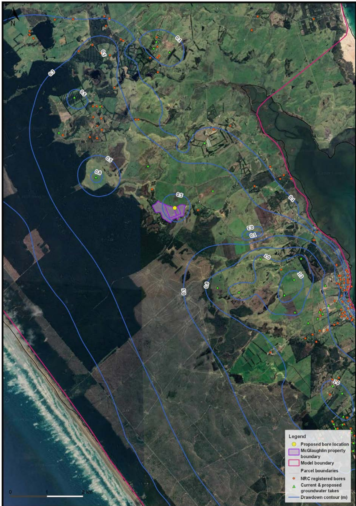
Figure 8. Cumulative drawdown (Scenario 2) in the shallow aquifer relative to a naturalised condition for all consented and proposed bores.
