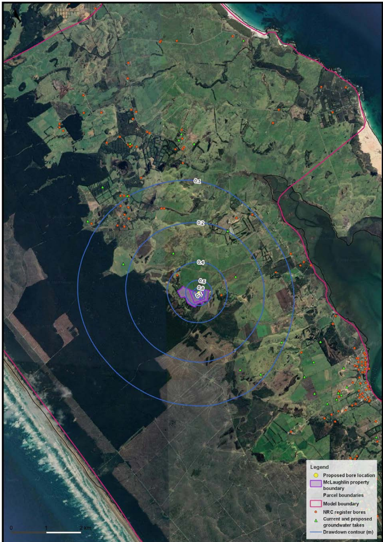
Figure 10. Simulated drawdown of deep aquifer resulting from proposed pumping at the McLaughlin bore (Scenario 3).
