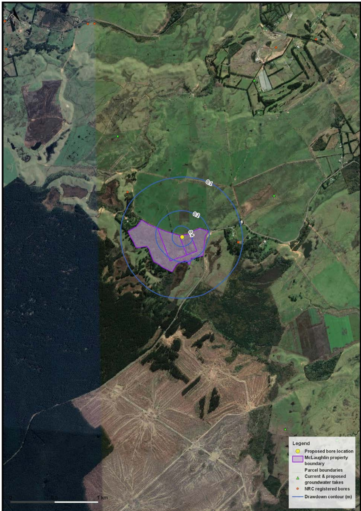
Figure 9. Simulated drawdown of deep aquifer resulting from proposed pumping at the McLaughlin bore (Scenario 2).
