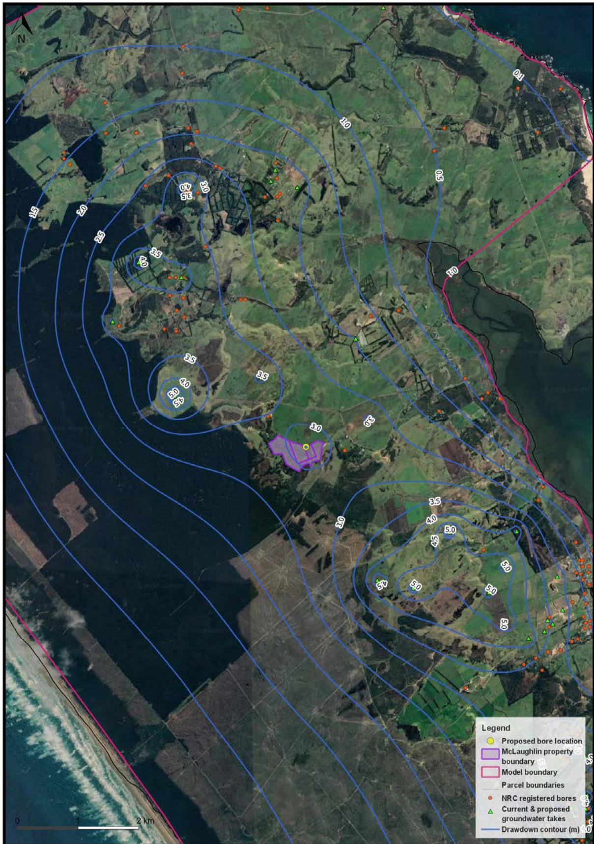
Figure 7. Cumulative drawdown (Scenario 3) in the deep aquifer relative to a naturalised condition for all consented and proposed bores.
