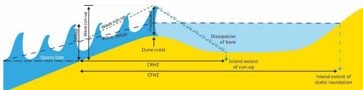
Figure 4-1: Definition sketch for CFHZ and CRHZ
