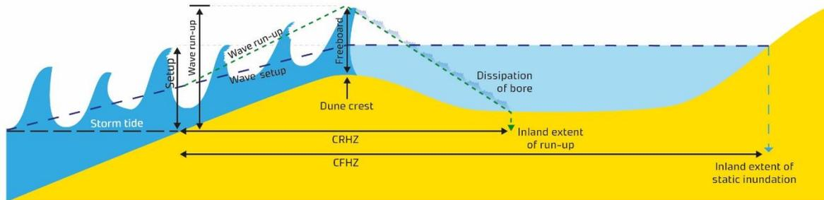
Figure 8-1: Definition sketch for CFHZ and CRHZ
