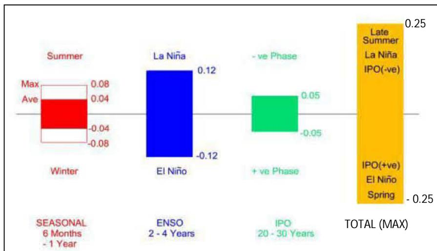
Figure 2-4: Components contributing to sea level variation over long term periods (source: MfE, 2008)
