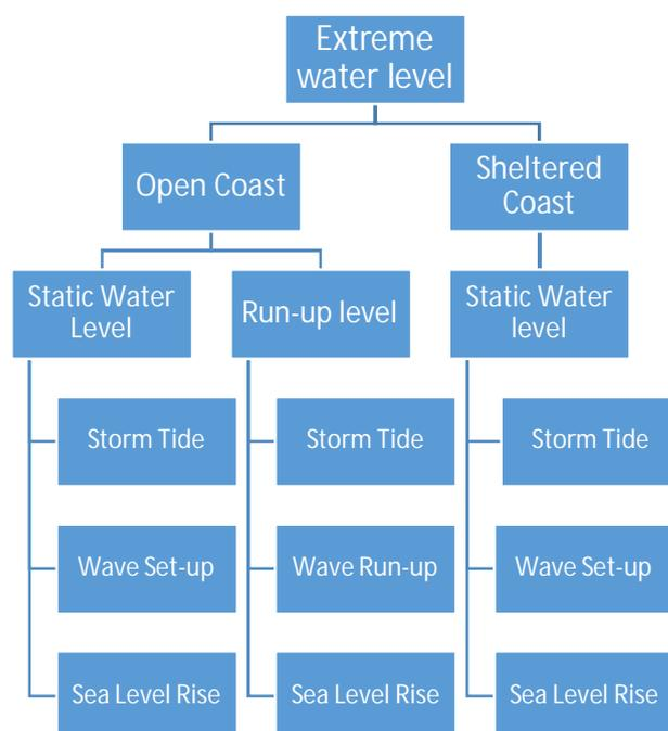
Figure 3.1: Extreme water level assessment diagram
