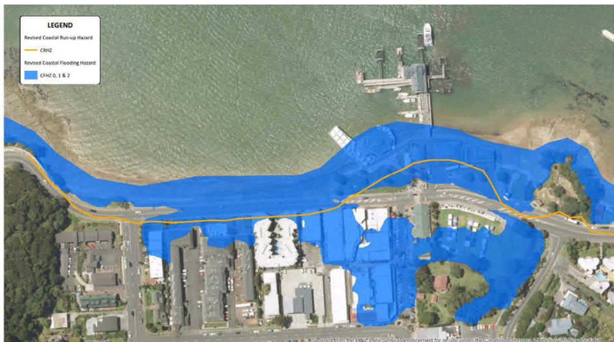
Figure 4-8: Revised CFHZ0/1/2 (blue polygon) and CRHZ2 (orange line) for Paihia CBD foreshore.
