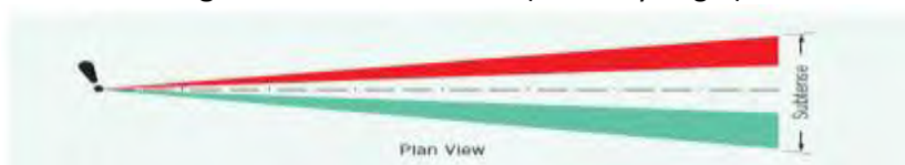
Figure 2 Light Sectors PEL (Courtesy Vega 5 )
