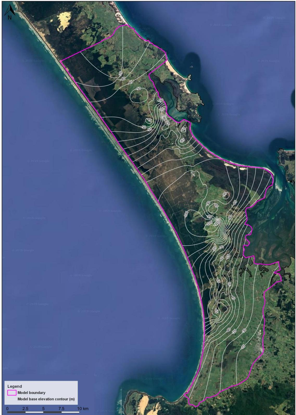
Figure 5. Model base elevation contours derived from bore log interpolation and 8m DEM data.
