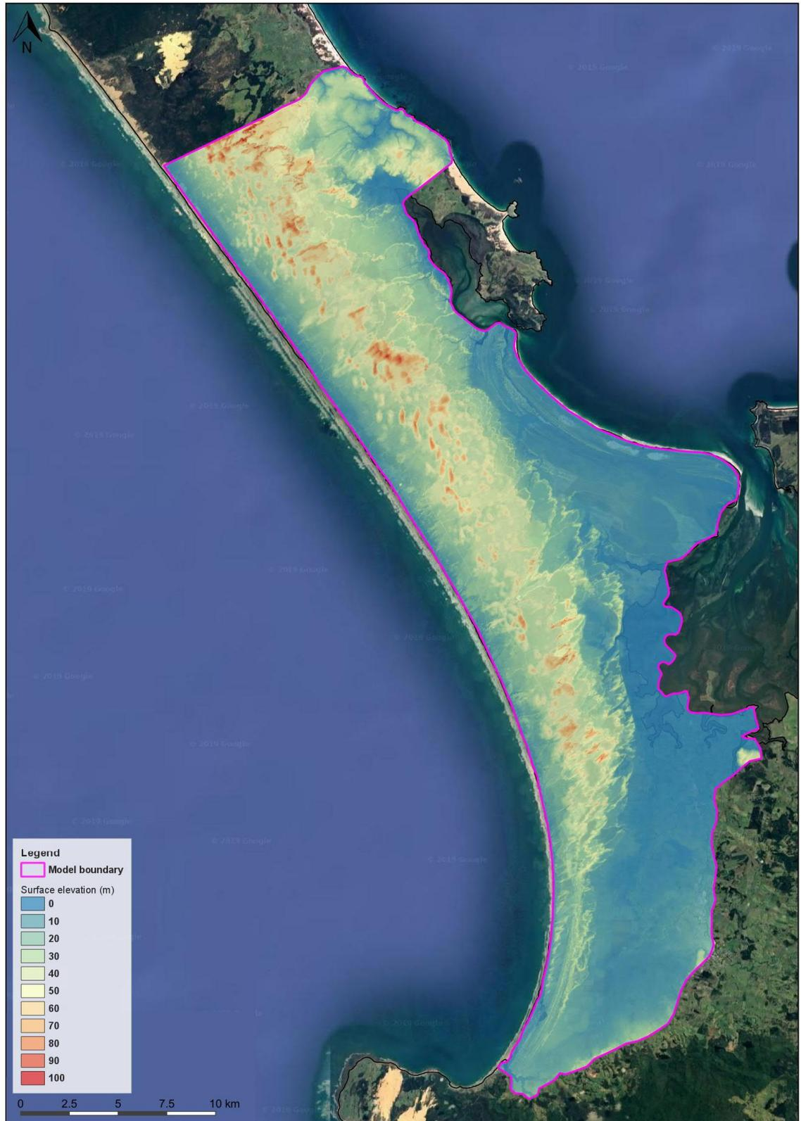
Figure 1. Surface elevation over AAGWM model area based on LIDAR survey.
