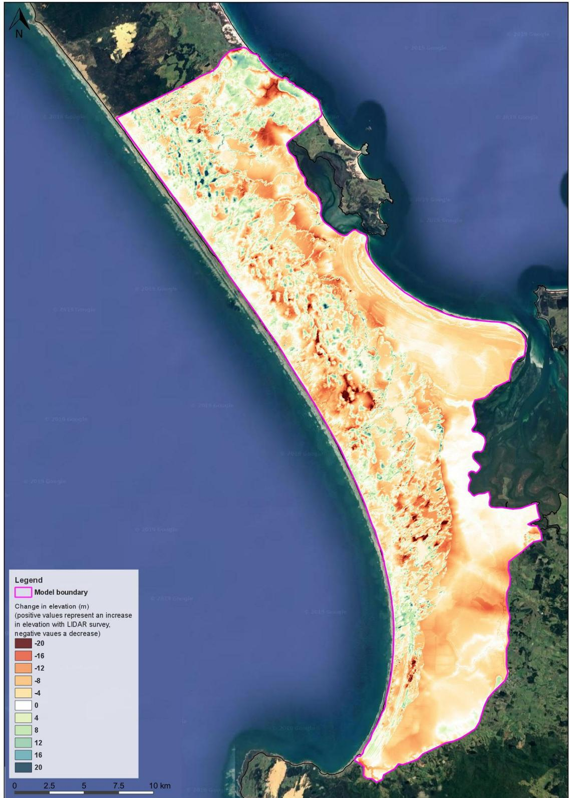
Figure 3. Difference in surface elevation (LIDAR – 8m DEM).
