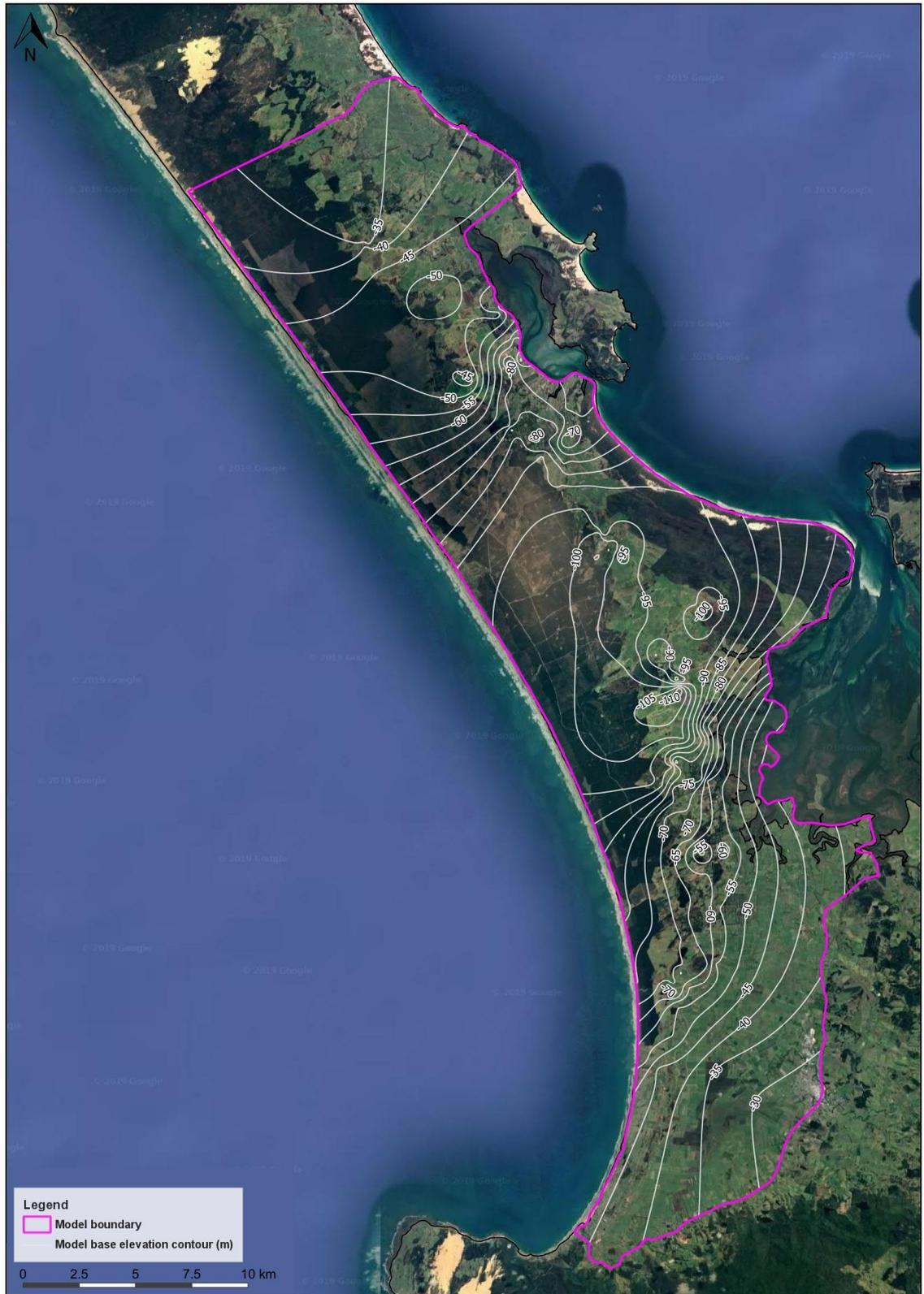
Figure 4. Model base elevation contours derived from bore log interpolation and LIDAR DEM data.
