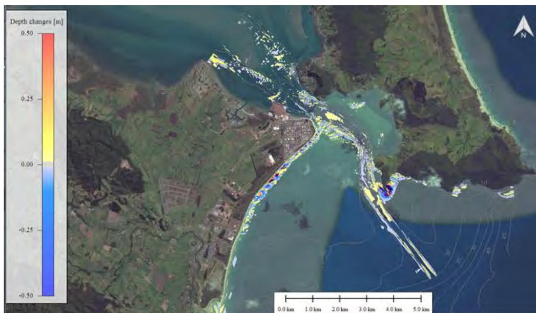
Figure 7.31 Changes in sedimentation and erosion patterns over the study area between the existing and post-deepening configurations over a 21-day sequence of storm and fair weather conditions.
