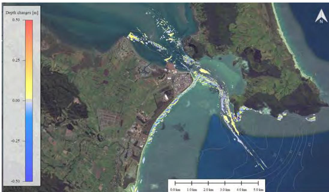
Figure 7.29 Changes in sedimentation and erosion patterns over the study area between the existing and post-deepening configurations over a 16-day fair weather event.
