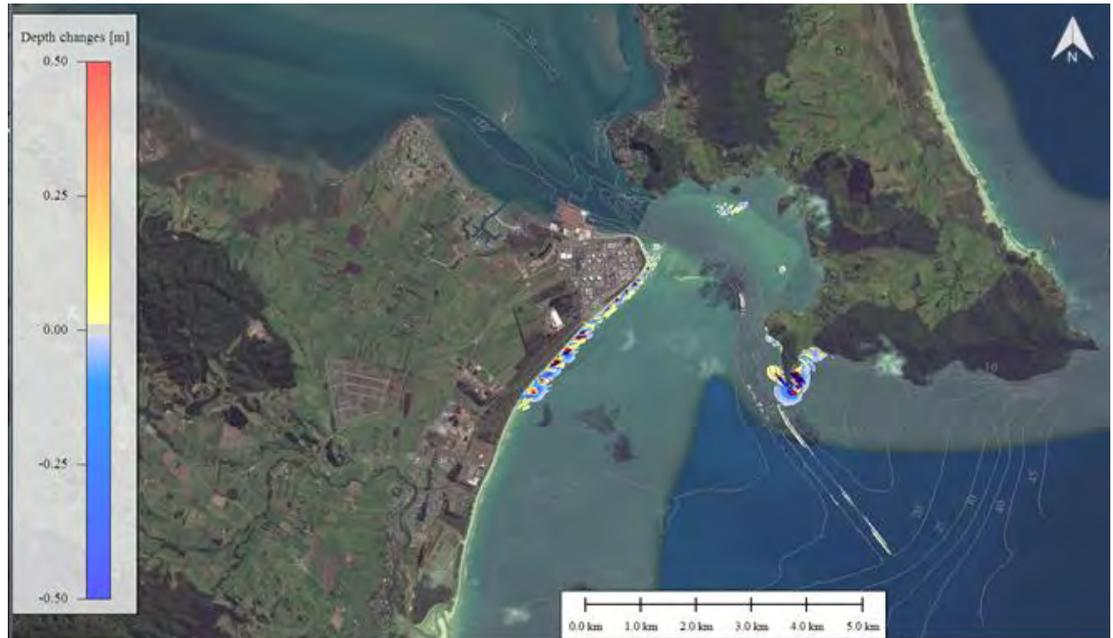
Figure 7.27 Changes in sedimentation and erosion patterns over the study area between the existing and post-deepening configurations over a 5-day storm event.
