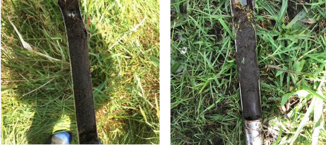
Figure 9: Soil core samples taken on Site 1 in October 2021, showing peat and sand composition
