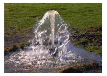
Photo: Overflowing artesian bore
