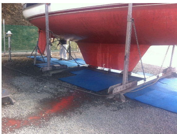
Plate 9. Discharges from wet sanding to remove old antifouling paint from a vessel's hull can be a source of metal contamination.
