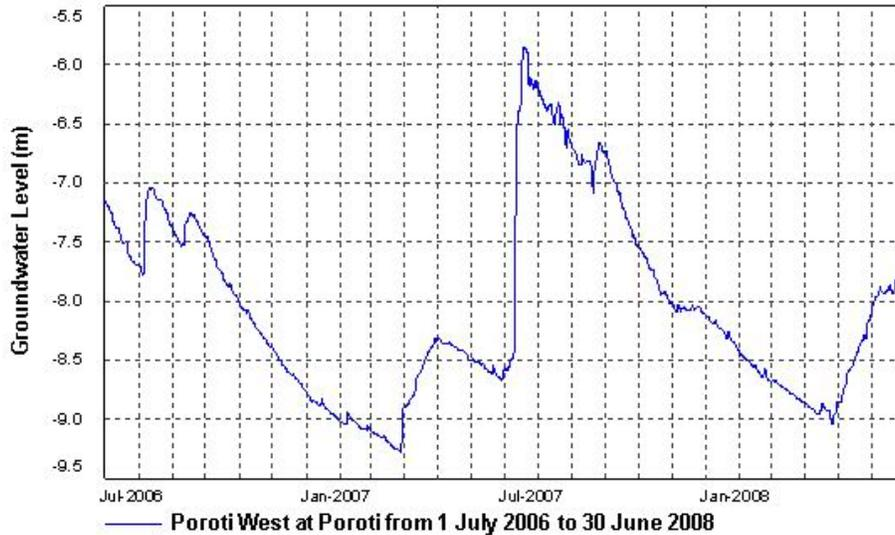
The groundwater recharge resulting from the two significant rainfall events in March and July 2007 can clearly be seen, with an increase in groundwater level of approximately 0.8 metres and 2.5 metres respectively. Groundwater levels began to increase within 24 hours of the rainfall events commencing.
