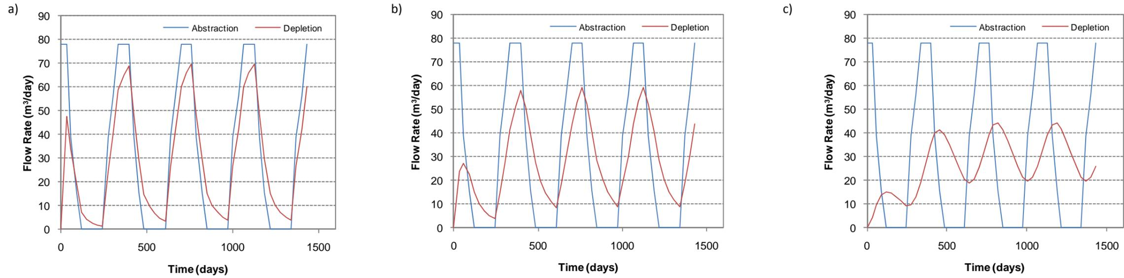
■ Figure 19. Abstraction and depletion rates for fractured basalt underlain by hard basalt with a) 35 m bore displacement, b) 200 m bore displacement and c) 1000 m bore displacement.
