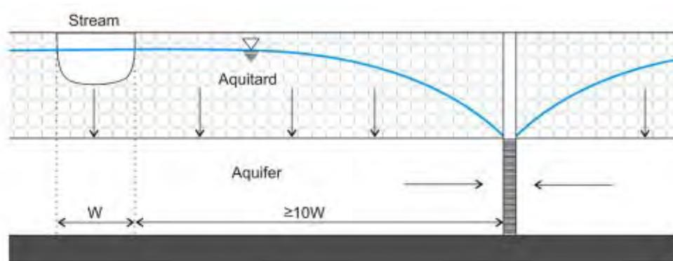
■ **Figure 5. Hunt (2003) stream depletion schematic.**
