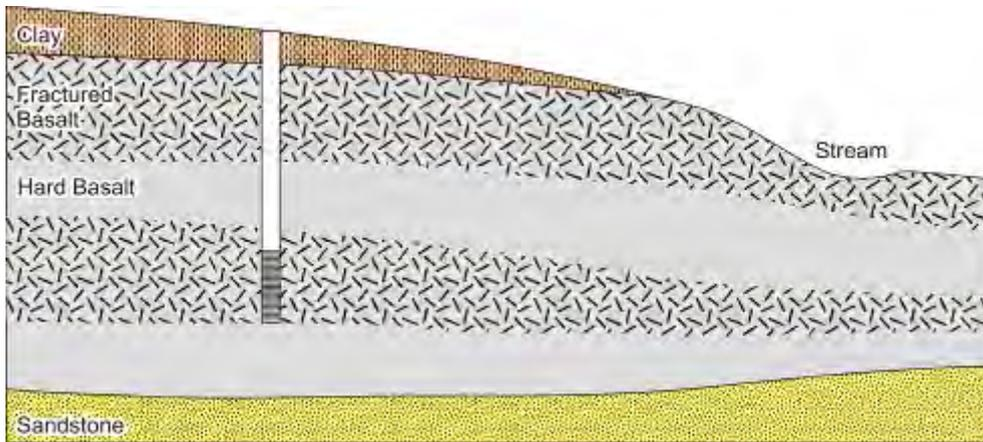
■ Figure 14. Layers of fractured and hard basalt.
