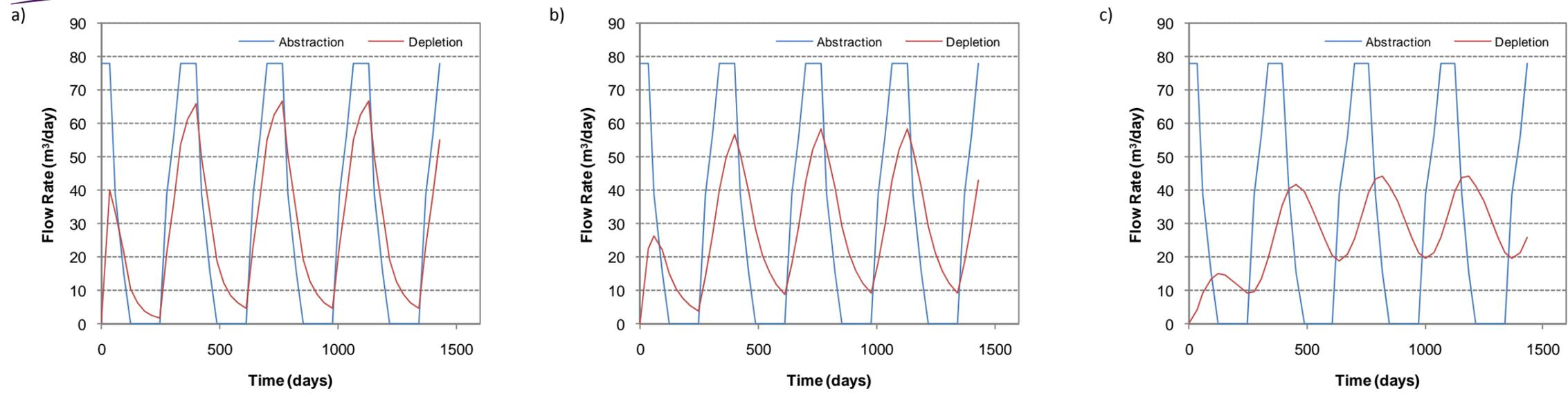
■ Figure 21. Abstraction and depletion rates for fractured basalt underlain by hard basalt with a fractured basalt zone with a) 35 m bore displacement, b) 200 m bore displacement and c) 1000 m bore displacement.
