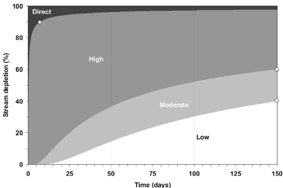
**Figure WQN5: Hydraulic connection categories for the management of stream depletion effects**
