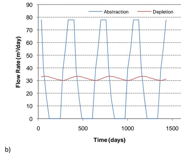
■ Figure 22. Abstraction and depletion rates for hard basalt with a scoria zone with a 200 m bore displacement.
