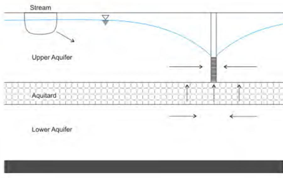
■ **Figure 10. Hunt (2009) stream depletion schematic.**
