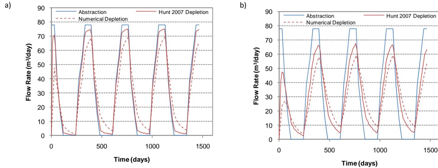
■ Figure 27. Stream depletion rates for numerical and Hunt (2007) analytical methods for fractured basalt underlain by hard basalt with: a) 35m bore displacement, and b) 200 m bore displacement, with a boundary at 800 m.
