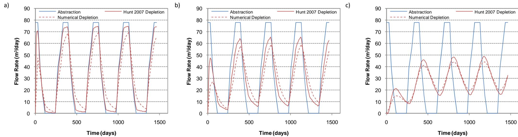
■ Figure 28. Stream depletion rates for numerical and Hunt (2007) analytical methods for fractured basalt underlain by hard basalt with: a) 35m bore displacement, b) 200 m bore displacement, and c) 1,000 m bore displacement with a boundary at 1000 m.
