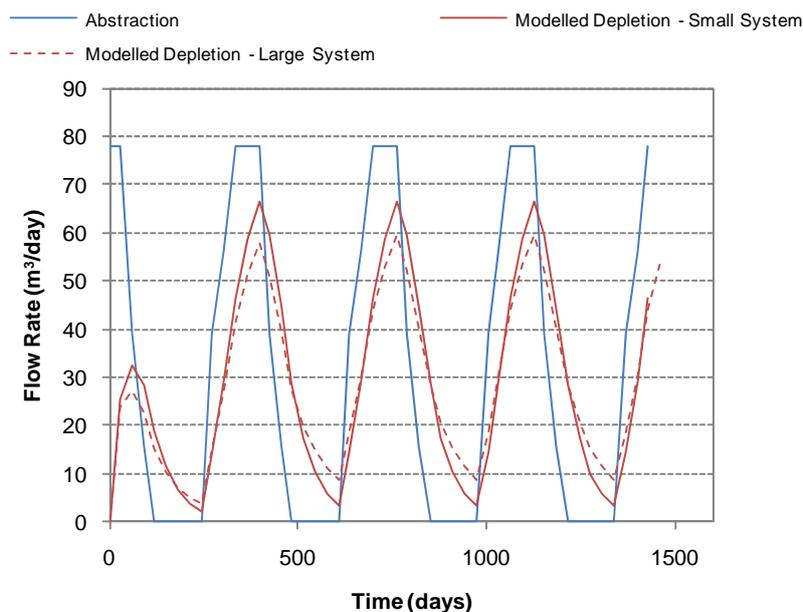
■ **Figure 25. Stream depletion with varying model domain (200 m bore displacement).**
