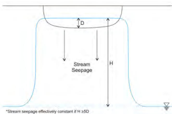
■ **Figure 2. Hunt Flow Net Analysis schematic.**
