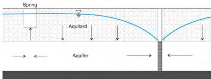
■ **Figure 11. Hunt and Smith (2008) spring depletion schematic.**
