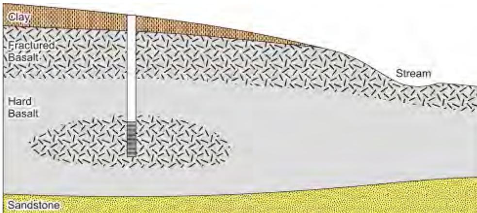
■ Figure 15. Fractured basalt underlain by hard basalt with a fractured basalt zone.
