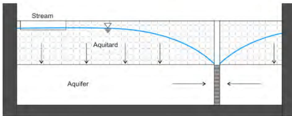
■ **Figure 6. Hunt (2007) stream depletion schematic.**
