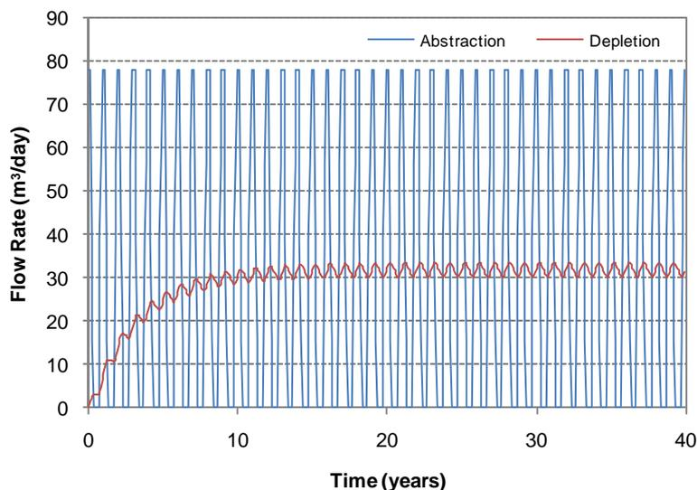
■ **Figure 24. Stream depletion for hard basalt with a scoria zone (200 m bore displacement) over a period of 40 years.**
