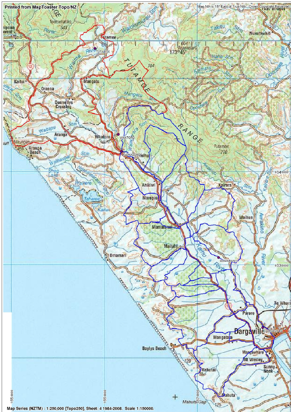
Figure 1: Kaihu catchment plan, upper catchments in red, lower catchments in blue. Rain and flow gauge locations also shown in purple.
