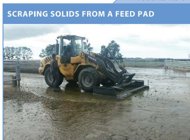
Washdown options include hoses or flooding systems. Figure 4.3-2 shows a flood system in operation. Flooding and hosing use comparable amounts of water, (flooding slightly less than hosing). The volume of water required will be reduced where solids are scraped off first (refer to Figure 4.3-3). A 3m wide scraper blade is quick and effective.
