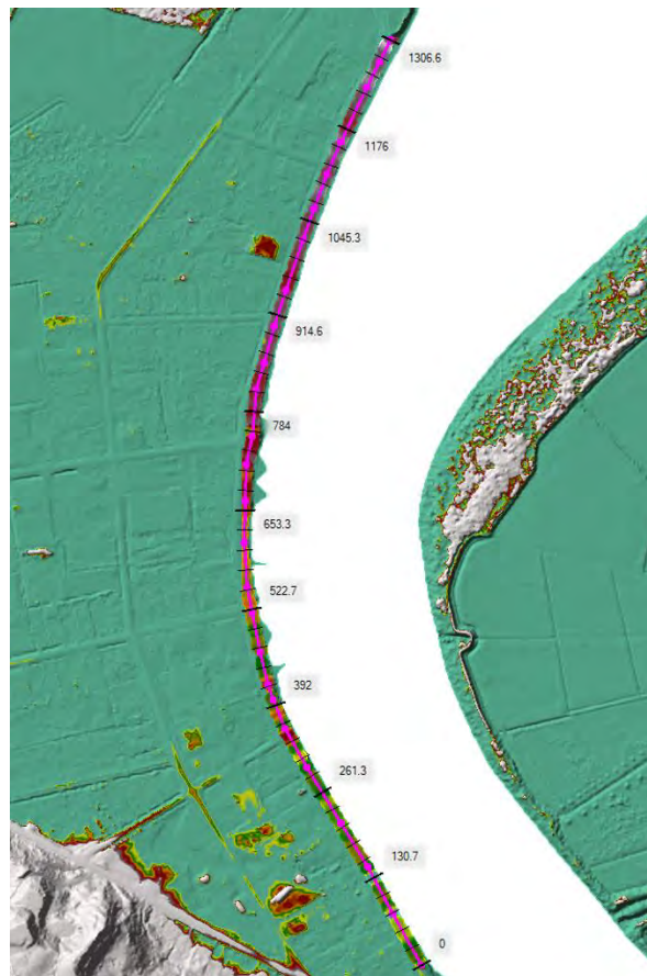
Figure 2.4. Kaihu-Dargaville DTM with pink line showing the location of the timber flood wall survey. Dargaville town is immediately landward of the stopbank.
