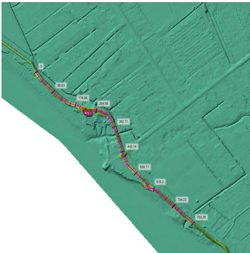
Figure 2.6. Ruawai DTM with pink line showing the location of the stopbank survey. Ruawai town is immediately landward of the stopbank.
