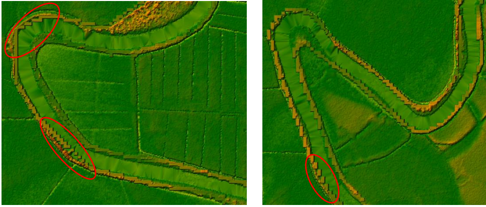
Figure 2.8. Gridded DTM of stopbanks overlain upon LiDAR at two locations along the Awanui River showing spatial inaccuracies (red circles) and general blockiness/staircasing.
