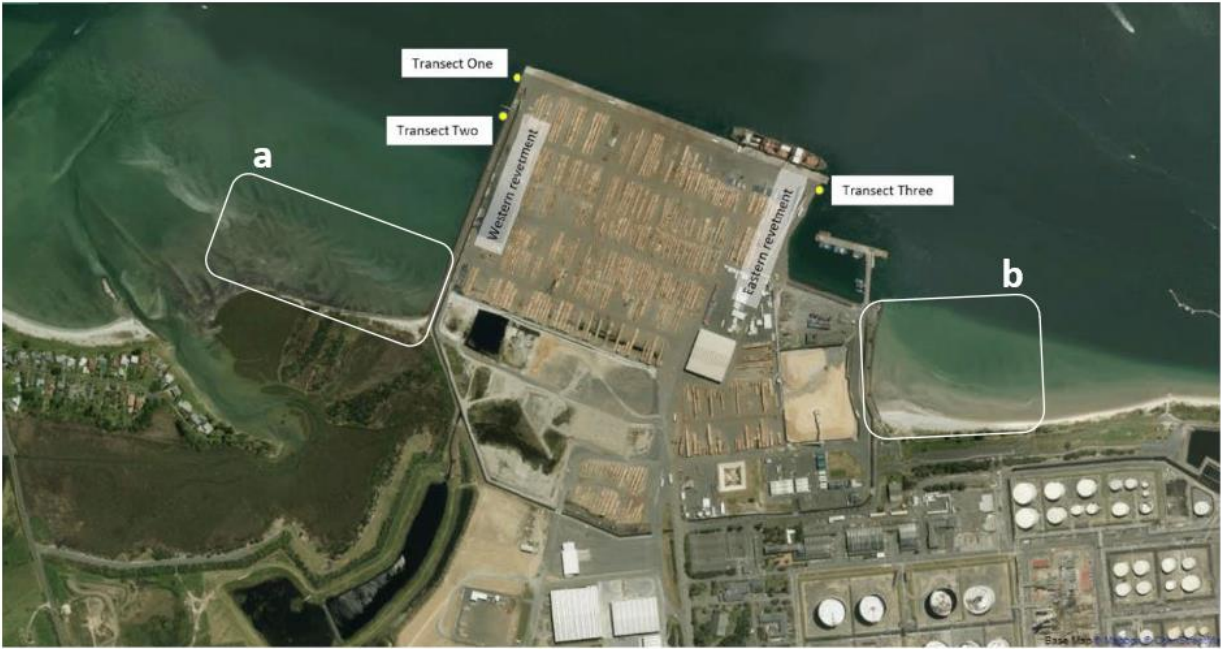
Figure Error! No text of specified style in document.. Evidence suggestive of sediment trapping by Northport structures along the southern shore of Whangarei Harbour. Annotation of Figure 19 from Poynter 2021a [9]. Area (a) shows area of organic matter/algae/seagrass detritus retention to the left of the western revetment. Area (b) shows area of sand build-up and shoreline progradation next to the eastern revetment.
