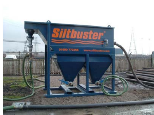
Photo 4: Lamella, or inclined plate, clarifier
